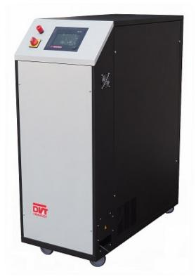
DETERMINES RESISTANCE TO PRESSURE OR BURST VALUE OF PVC, POLYRPROPYLENE, POLYETHYLENE ETC. PIPES
